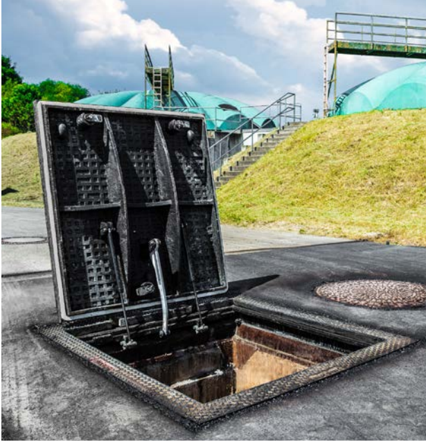
Surface-water-tight cast-iron cover with an opening aid, a load class of D 400 and a clear opening of 1000 mm x 1000 mm, Munich
